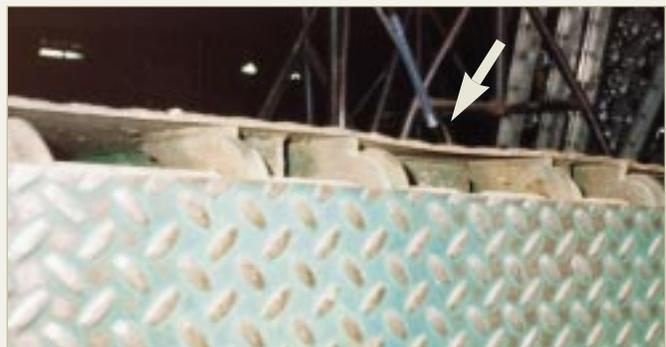
**Inadequate capacity can cause structural failure.** This photo shows how a leveler can bow, or "dish," when its capacity cannot handle the weight of the loads it must support.
