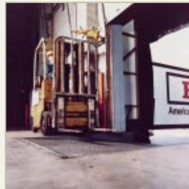
*A dangerous void in the floor is created when the leveler does not automatically return to dock height.*
