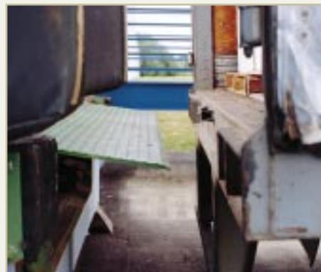
*Inability to retract lip can cause damage to cargo or equipment.*
