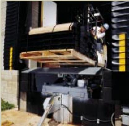
*Hydraulic velocity fuse free-fall protection.*
