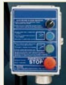
**WARNING:** Don't use an emergency stop button in place of a solid support strut to hold the leveler up during maintenance. This system is not designed to support extreme weights, such as a forklift turning onto the leveler. Plus, if power is lost for any reason, the leveler can drop.
