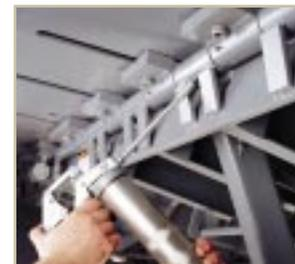
*Convenient grease fittings simplify lubrication.*
