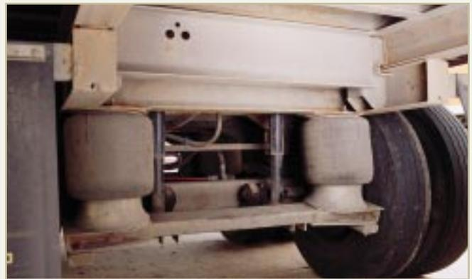
**Air-ride suspensions.** More and more air-ride trailers are being used today. They improve driver comfort and help protect cargo. But unless specially equipped, the air must be released when the truck is parked at the dock to help prevent "trailer walk" and ensure safe loading and unloading. The release of air can lower the bed height as much as 8", meaning you'll need a longer leveler to safely service these trailers.
