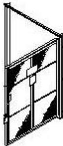
opening width is limited normally to approximately 60” to 72” maximum and requires clear space in front of the lift to swing open.
